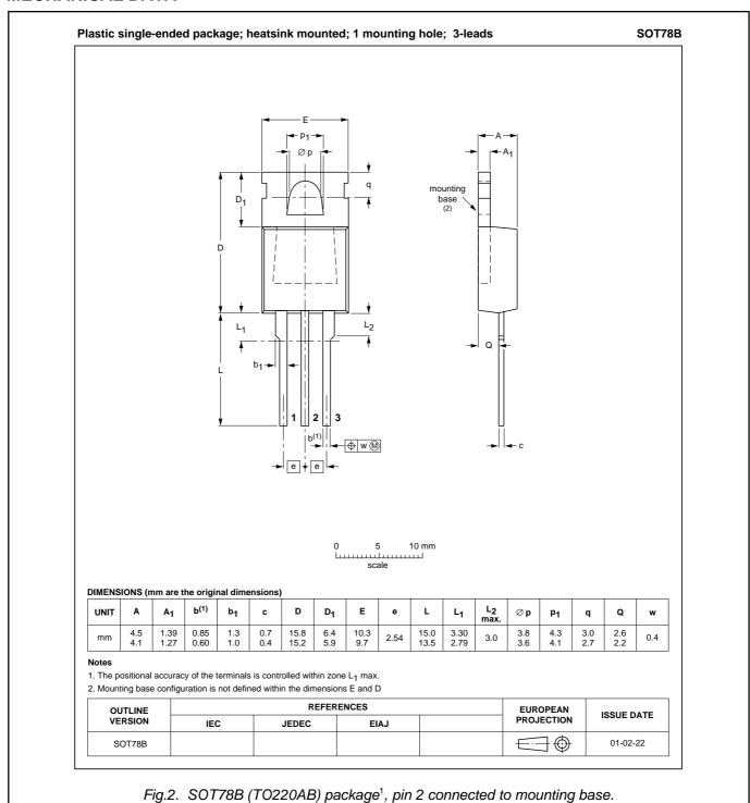
1 Refer to mounting instructions for SOT78 (TO220) envelopes. Epoxy meets UL94 V0 at 1/8". Net mass: 2 g
